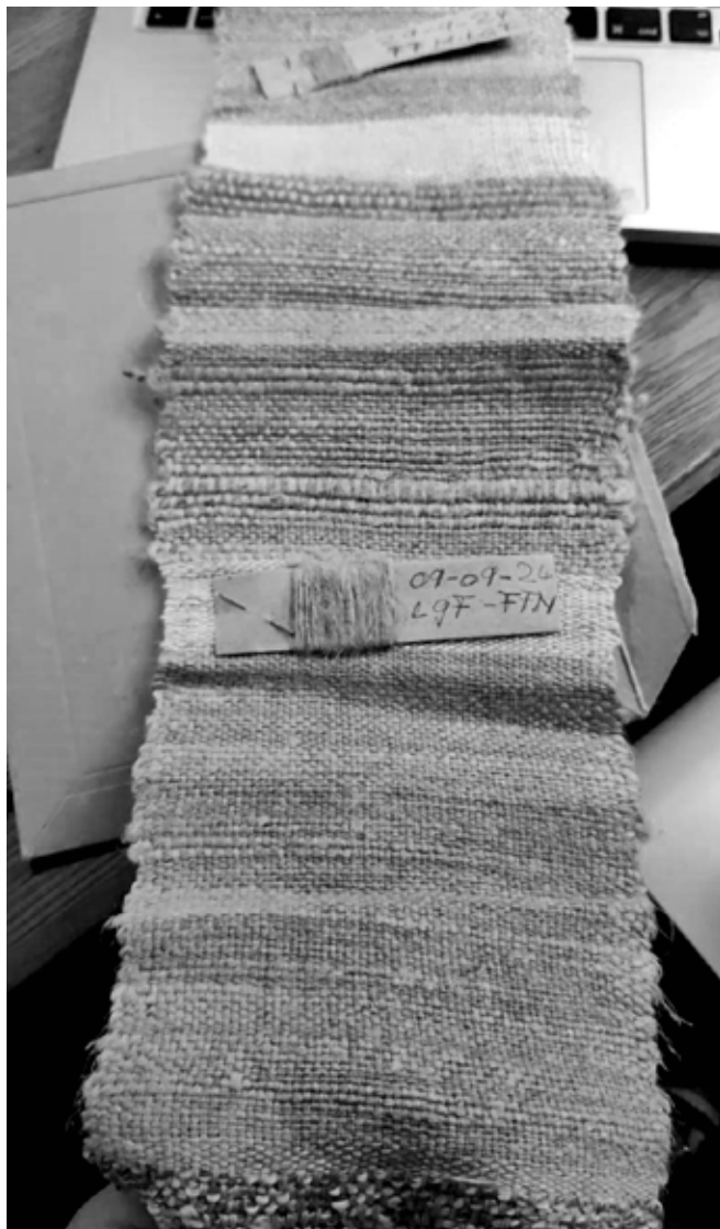
Left and Above: A sample weaving showing the progression of yarn quality development through the evolution of the spinning machine's design. Bottom to Top: Yarn with slubs left in, Improved yarn without slubs, Control sample of commercial yarn.
